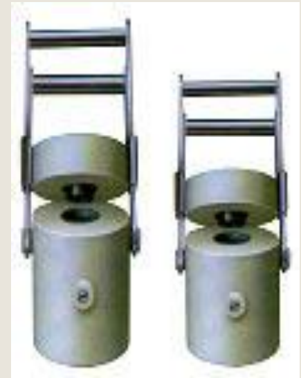
Lead pigs are used to store radiation sources
