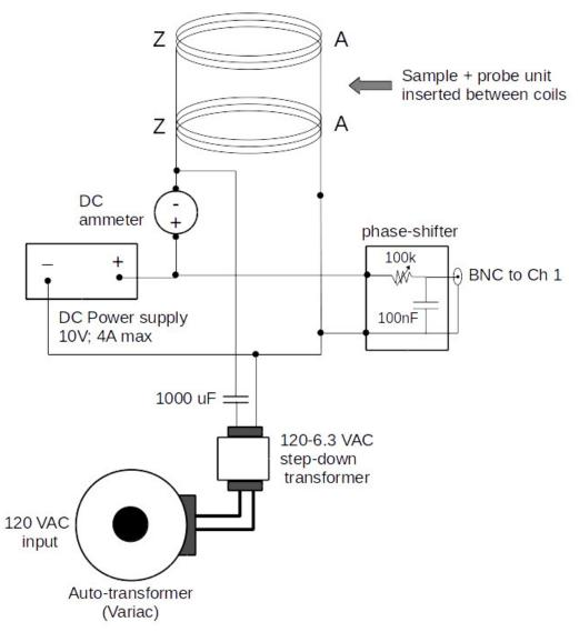
Figure 1: Connect the Helmholtz coils ( $2R=13.5~{\rm cm}$ ) in parallel and separate them by a distance R. The probe unit (see Figure 2) should fit snugly between the two coils. Set the AC voltage on the secondary winding of the step-down transformer to  $\sim 2~{\rm Vrms}$ . Do not exceed 2A DC into the individual coils, or 4A total.
