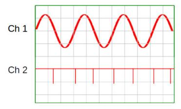
Figure 3: Representative oscilloscope waveforms. The top trace shows the current in the Helmholtz coils. The lower trace is the RF probe signal; distinct spikes identify resonance. DC current, RF frequency, and phase should be carefully adjusted to put the resonance points exactly at the crossovers of the sine wave.
