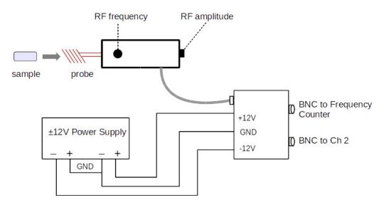
Figure 2: Connections of the probe unit, adapter, and split-mode power supply. The sample is inserted into one of three different probe solenoids. Drawing not to scale.
