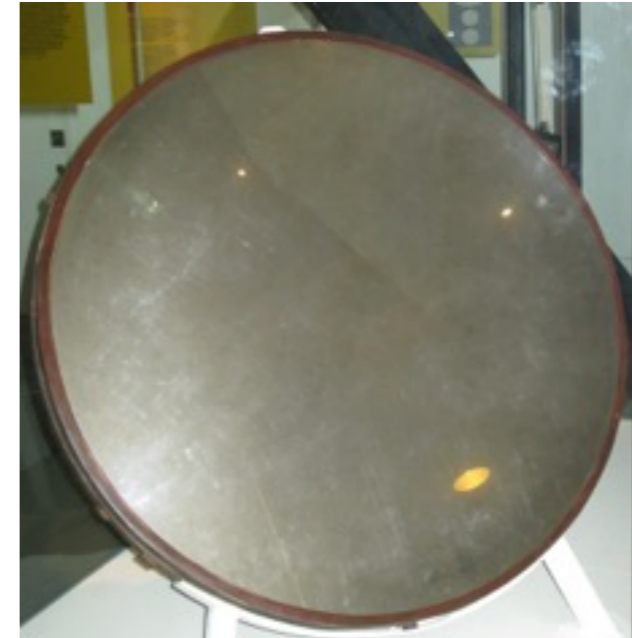
Herschel's telescope primary mirror (1.26m) (1875-1879)
